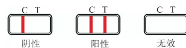
图 1 肺炎链球菌抗原检测试纸条结果判定 Fig. 1 Result interpretation of Streptococcus pneumoniae antigen immunochromatographic strip
