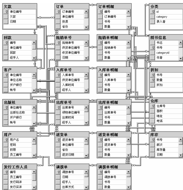
图4 数据库表与表间关系图 Fig.4 Relationship diagram between database tables
